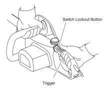
Figure 10 - Lockout Button and Trigger Location
